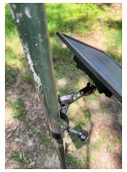
Repeat above steps to mount and align M.I.N.E.® Photo Camera on T-Post.
