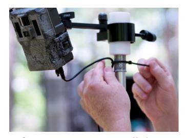
Turn on camera and allow time for connection to cellular network. Ensure all three battery icons appear in bottom right; Solar Panel, AA and Lithium.
