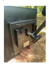
Lower round collar over T-post spine and position between two studs at least 12-inches from top with JAGER PRO logo and power ports facing the ground. Tighten collar thumb screw against T-post spine to secure mount with three contact points. Move 4-inch mounting arm south by loosening arm thumb screw. Align solar panel by loosening ball compression screw and tilting to proper angle. Tighten both arm thumb screw and ball compression screw to secure solar direction and angle.
