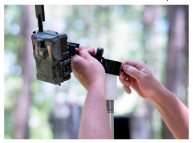
Move 4-inch mounting arm towards feeder by loosening arm thumb screw. Align camera by loosening ball compression screw and tilting to proper angle. Tighten both arm thumb screw and ball compression screw to secure camera direction and angle.
