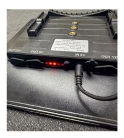
First red LED will flash while batteries are between 0 and 24% charged.
