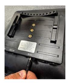
Plug USB port into an AC outlet adapter.
