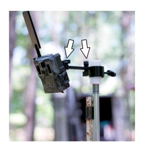
Insert one end of the 10' long, 12-volt cable plug into the lithium battery 12-volt port and insert opposite cable plug into the camera DC port then secure to extended pole with a zip tie.
