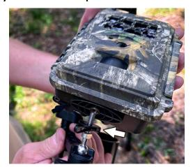
Lower round collar over nylon adapter and position between top two studs with JAGER PRO logo and power ports facing the ground. Tighten collar thumb screw against nylon adapter to secure mount with three contact points.
