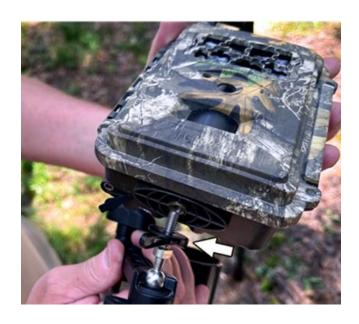
Insert one end of the 3' long, 6-volt cable plug into the lithium battery 6-volt port and opposite cable plug into the I.C.E.® Camera DC port.
