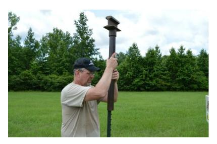
Measure and mark 12 inches with a permanent marker on both sections of a 12-foot-long extended pole. These marks ensure maximum camera height will be ten feet when finished with one foot below locking tabs in each section for maximum strength.
