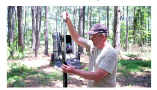
Rotate extended pole until feeder and both gates are centered in the camera field of view.
